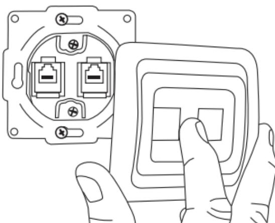
Install the mechanism into the hollow in the wall, tighten firmly the locking and the fastening screws on the unit housing. Install the decorative frame and the cover.
